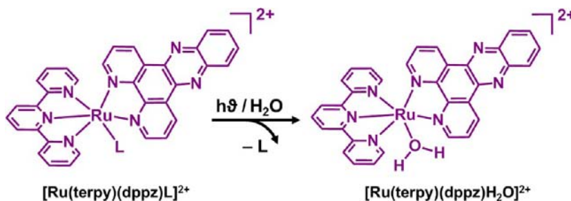
Figure 1. Photochemical activation of ruthenium(II) polypyridyl complex. The monodentate ligand (L) is photoexpelled from the ruthenium(II)–dppz complex on irradiation with visible light.
